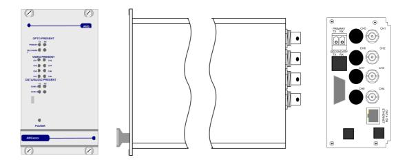
The **AMG4641ER** is a rackmount four channel video transmit unit designed to transmit 4 video signals and provide full duplex 100BaseT Ethernet connectivity over two Multimode fibres.
